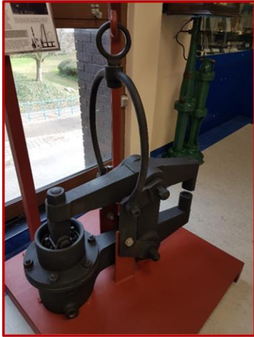
Hydraulic Riveting Machine – William Arrol circa 1888
