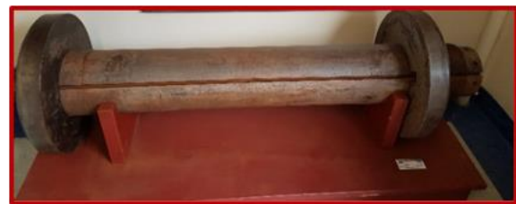
Forth Bridge Original Pin Assembly – Circa 1890
