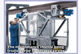
The maintenance shuttle being trialled prior to delivery to site
